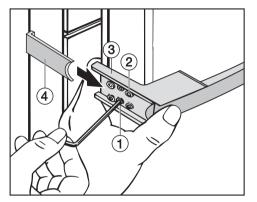
■ Loosely attach the handle to the opposite side of the door with the two front screws ②.
